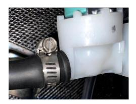
Wash motor requires a <u>6720595</u> clamp on the outlet side, and a <u>6736595</u> clamp on the inlet side.
